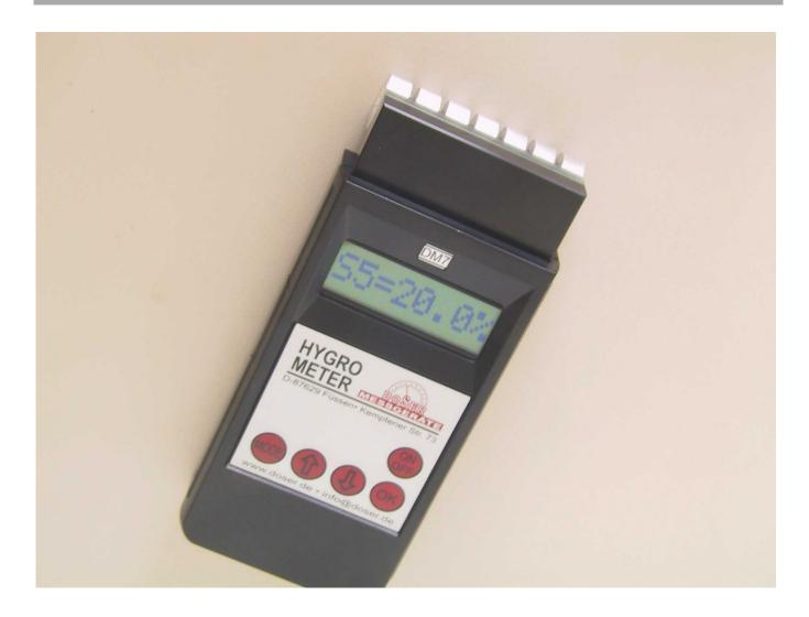
Moisture Meter type DM7 for veneers, corrugated boards, sigle card boards, cardboard pipes etc.
