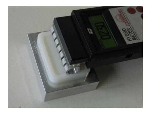
The test module PE35-7 can be used for testing and calibrating of our capacitive moisture meter DM7-AL and DS7U.
