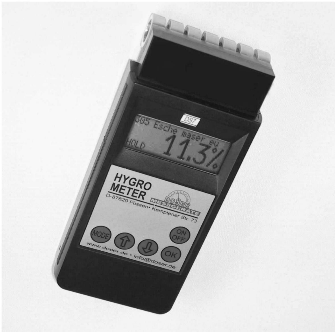
The DS7 can be used for measuring moisture in veneer piles
